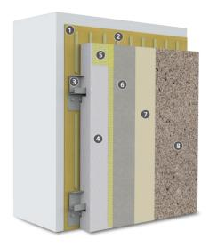
Structural Back-up Wall (by others): Steel or wood frame with glass mat gypsum sheathing in compliance with ASTM C1177 or code compliant OSB or plywood sheathing, concrete or concrete masonry, existing strucuturally sound, uncoated brick or other masonry wall construction.
