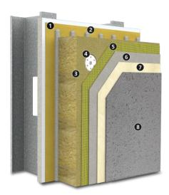
Substrate (by others): Glass mat gypsum sheathing in compliance with ASTM C1177, code compliant OSB or plywood sheathing, concrete or concrete masonry, existing strucuturally sound, uncoated brick or other masonry wall construction.
