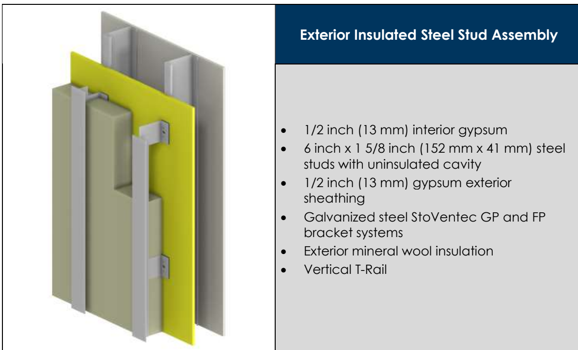
Figure 1.1: Schematics of Evaluated StoVentec Galvanized Steel GP Assembly
