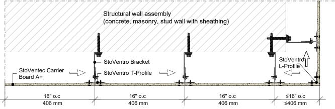
StoVentro<sup>™</sup> Wall Brackets and T-Profile alignment and requirements at outside corners, jambs and returning transitions.
