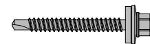
StoVentro Steel Stud Fastener 1/4" -14 x 2" self-drilling hex head screw with washer - (stainless steel)
