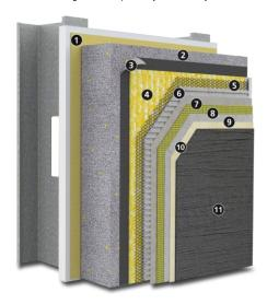
Substrate: Glass mat gypsum sheathing in compliance with ASTM C1177, Exterior or Exposure 1 wood-based sheathing (plywood or OSB), code compliant concrete or concrete masonry wall construction.
