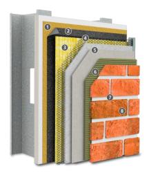
Substrate: Glass Mat Gypsum sheathing in compliance with ASTM C1177, code compliant wood-based sheathing (plywood or OSB), code compliant concrete, concrete masonry, existing structurally sound, uncoated brick or other masonry wall construction.
