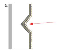
Excess base coat installed in reveal
