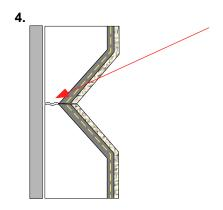
Less than 0.75" (20 mm) insulation behind reveal
