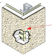
Damage to insulation, base coat and finish.
