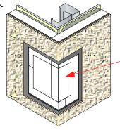
Insulation tightly fitted
