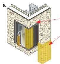
New base coat material installed with new mesh overlapping the existing
