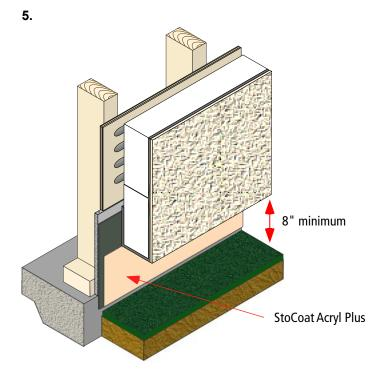
When the EIFS repairs are completed, the foundation may be coated with StoCoat Acryl Plus to provide a color match or accented finish over the Flexyl waterproofing.
