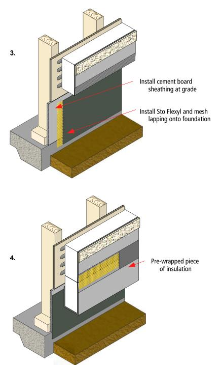
**3.** Install cement board to replace the sheathing removed. As the replacement EIFS will terminate higher above grade the previous installation, a band of sheathing will be left exposed. The cement board will be more durable than wood sheathing.
