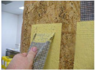
is grasped and pulled to provide an indication of the bond strength. The force required to complete the test combined with visual observation of the coating/substrate is the basis for conclusions about the test results. Some typical post-test observations and conclusions are:
